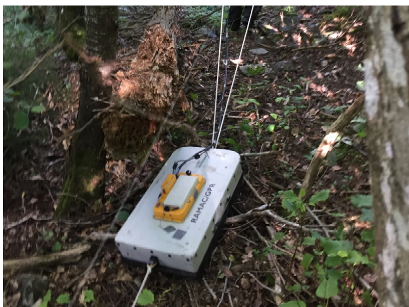
Figure 2 GPR 250 MHz antennae in action
